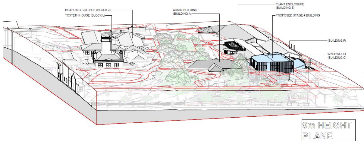
Figure 40: 3D Height plane diagram showing existing areas of height non-compliance and proposed area of non-compliance in blue
