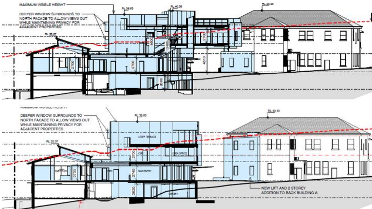
Figure 46: Section Plan (north-south) - Original submission top, amended submission below. Note the amendment to the internal levels which removes the half levels previously proposed, the reduction in built form adjacent to the Administration Building and rationalisation of the roof form.
